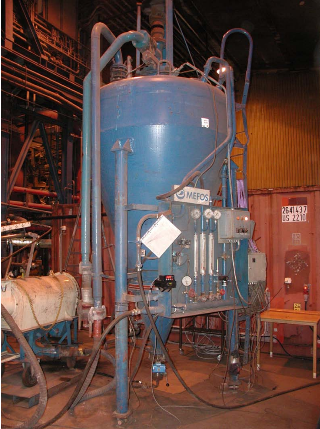
Figure 8, Coal injection lock hopper
