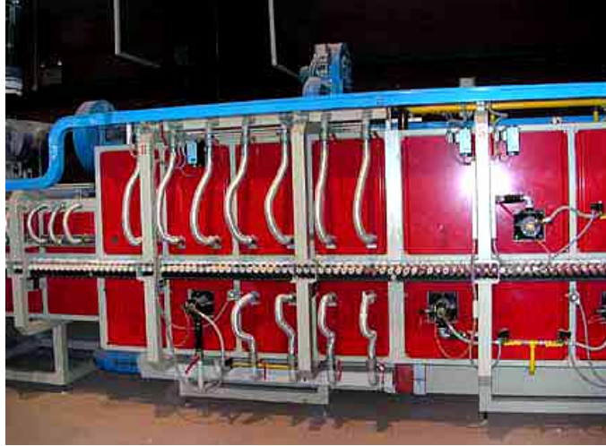
Fig 5. Firing zone of the kiln (gas burners below and above rollers)
