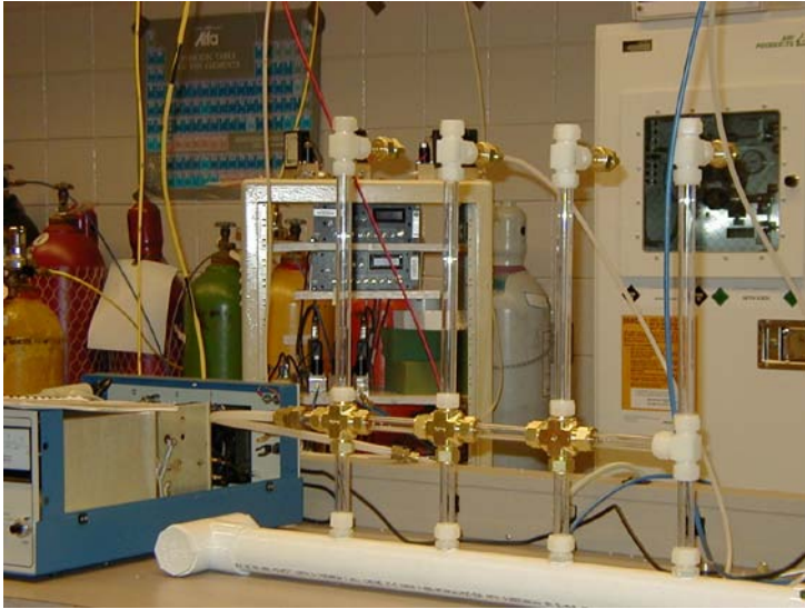
Figure 5: The picture of the plasma reactor. Shown are four identical stages in parallel.
