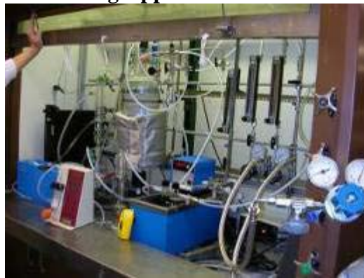
Figure 5 Mercury Vapor Sorption Apparatus
