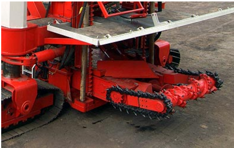
Figure 5. Anchoring Pins Used to Stabilize the Base Frame (Photo courtesy of SHM website).
