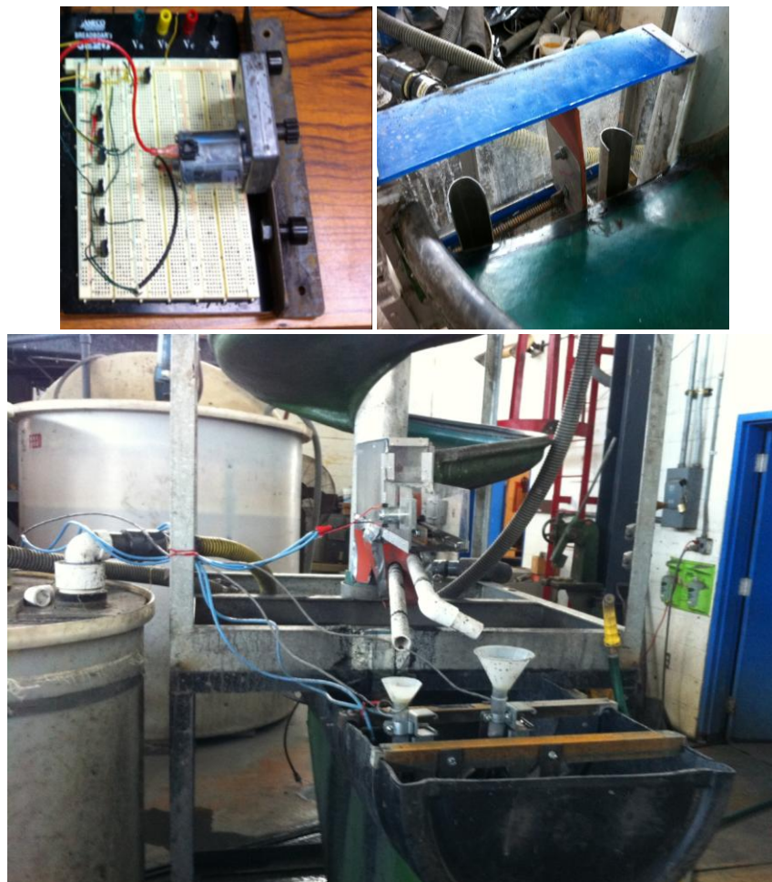
Figure 4: Components of the spiral automation system: PIC microcontroller (top left), splitter box (top right), and sensing tubes fed from splitter box (bottom).
