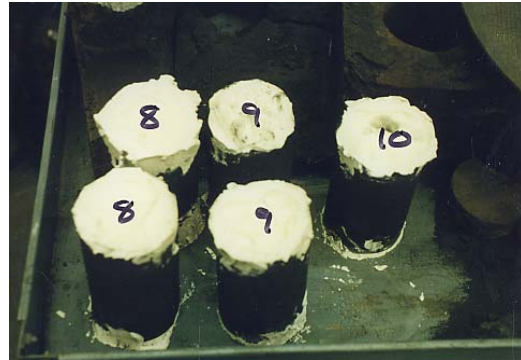
Figure 4: This tested depth of sintering of panel 9 from the second pour; the other panels from this pour had similar results.
