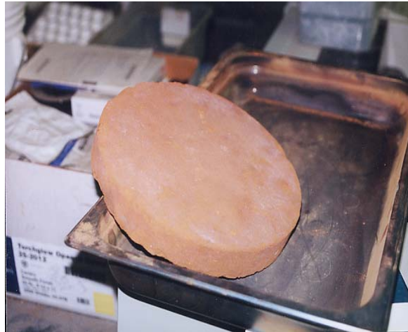
Figure 7: Compression disk made from panel 14 and 15 materials.
