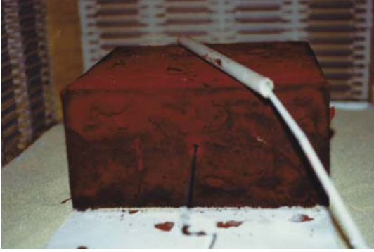
Figure 13: Block 1 fired at 700 °C (shown with thermocouples).
