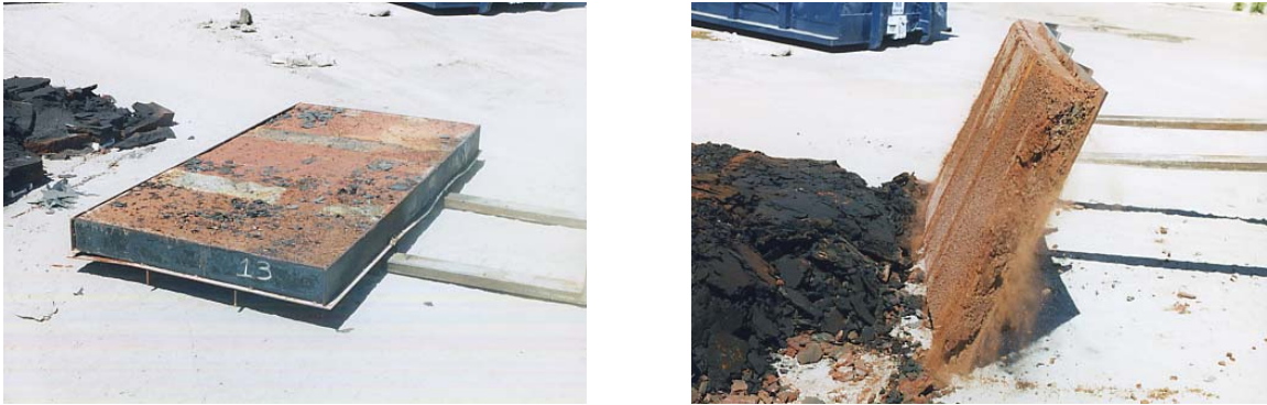
Figure 10: Panel 13 just before being dumped on left, note deformation in steel mold and loss of weld integrity; right: Panel 15 as it is being dumped off of the mold. This panel shattered into small pieces.
