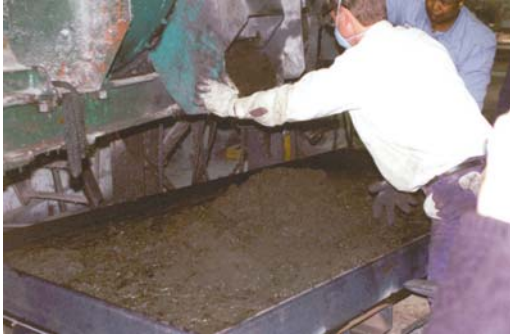
Figure 1. Full-scale panel being poured at Magneco Metrel.
