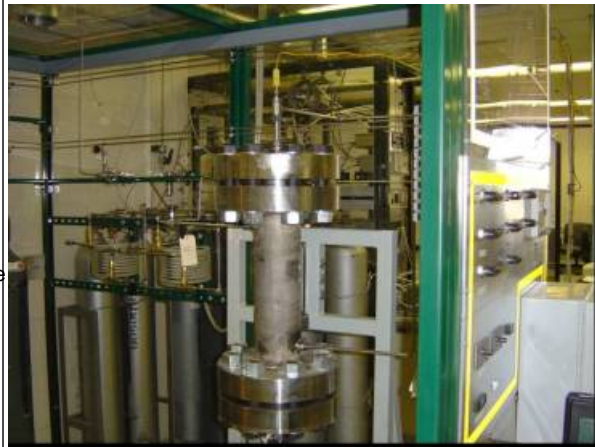
Figure 3. Photo of high temperature/high pressure membrane permeation unit
