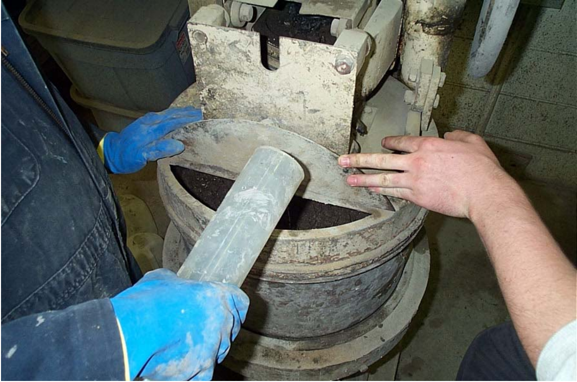
Figure 2. Counter-current pan mixer used for laboratory sample preparation.
