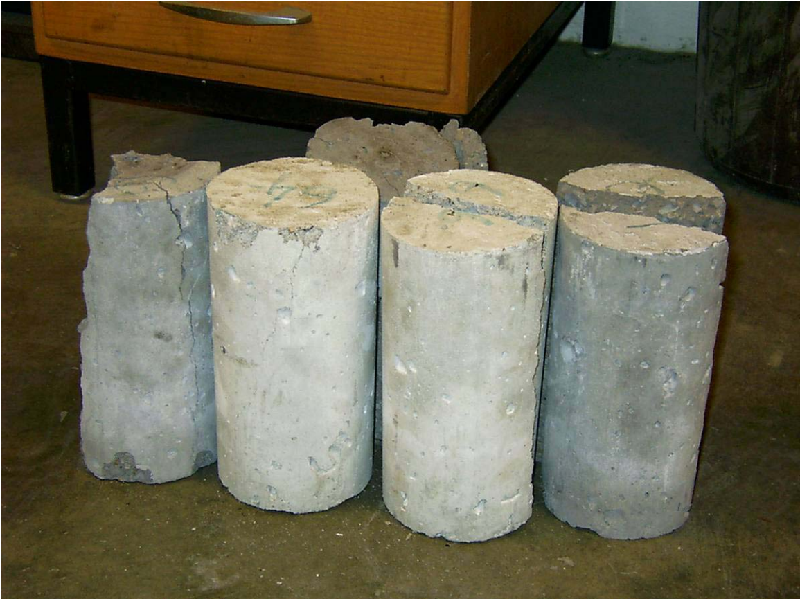
Figure 4. 6-inch x 12-inch laboratory samples tested for compressive strength and indirect tensile strength.
