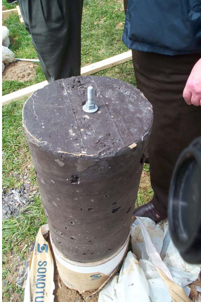
Figure 9. CCBs based foundation pier after 7-days curing time. Anchor bolt is visible on top.
