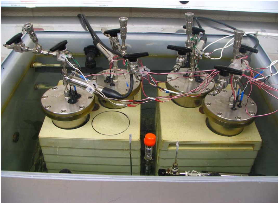
Figure 2: Constant temperature water bath with four the pressure vessels for volumetric strain measurement.
