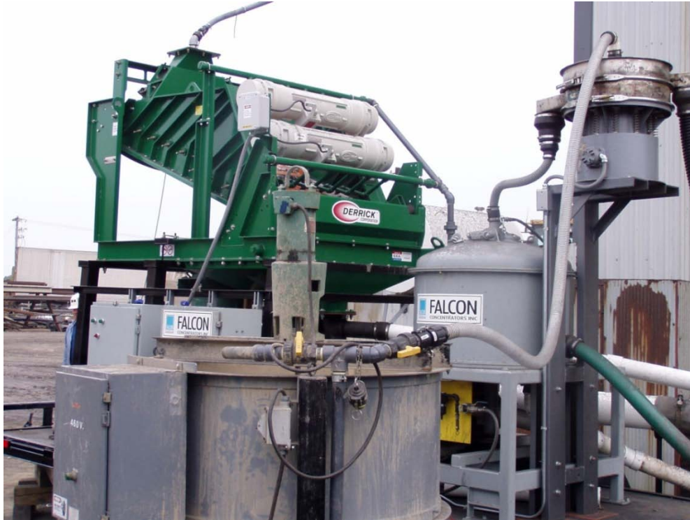
Figure 4: Single deck Stack Sizer and C400 Falcon Concentrator at Creek Paum Mine.
