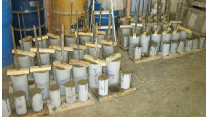
Figure 8. Cylindrical sample for bond strength testing of concretes
