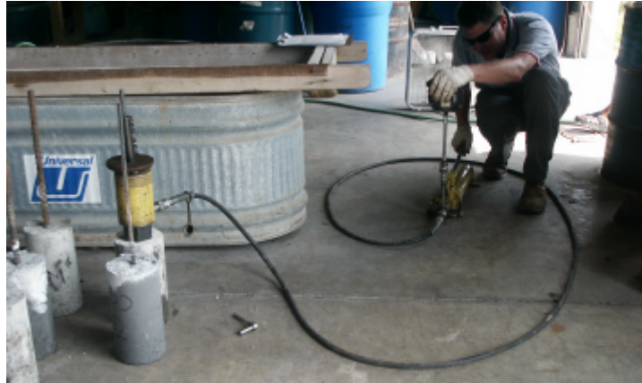
Figure 13. Bond strength of cylindrical samples in progress
