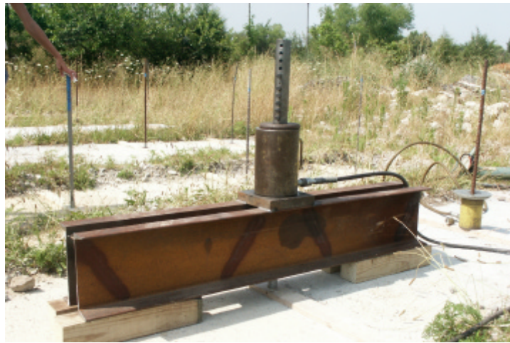
Figure 14. Bond strength testing of concrete in field trenches in progress
