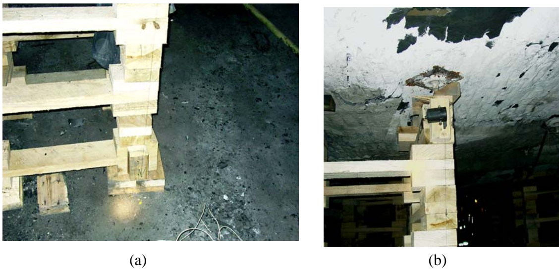
Figure 11: Wire extensometer attached to (a) bottom element, and (b) top element.
