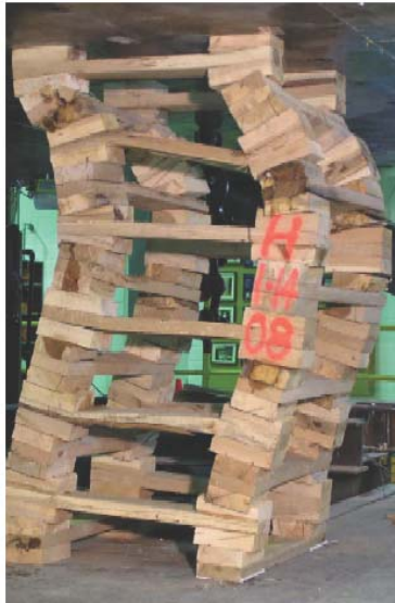
Figure 6: ATLAS series 100 severely arching due to differential loading.
