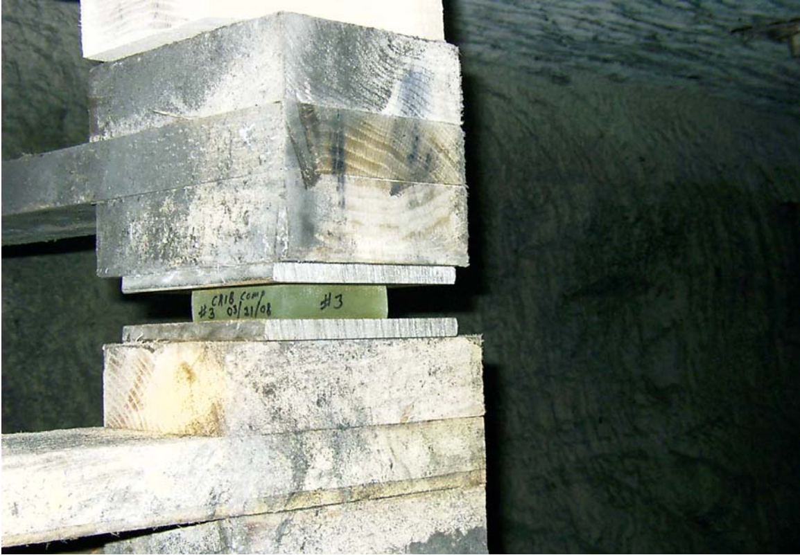
Figure 13: SIU developed load cell in one corner of an ATLAS crib.
