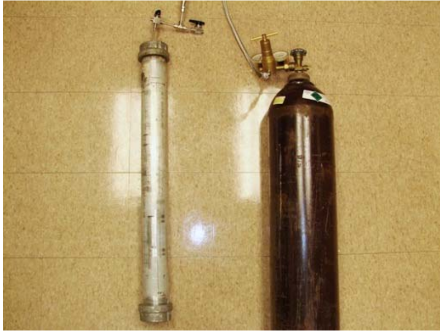
Figure 4: Setup for CT-Scan of coal cores.
