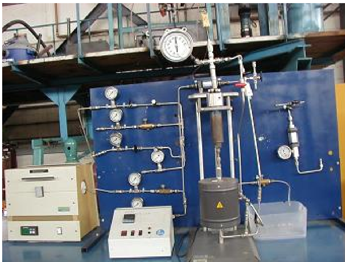
Figure 10. Reactor system set up.
