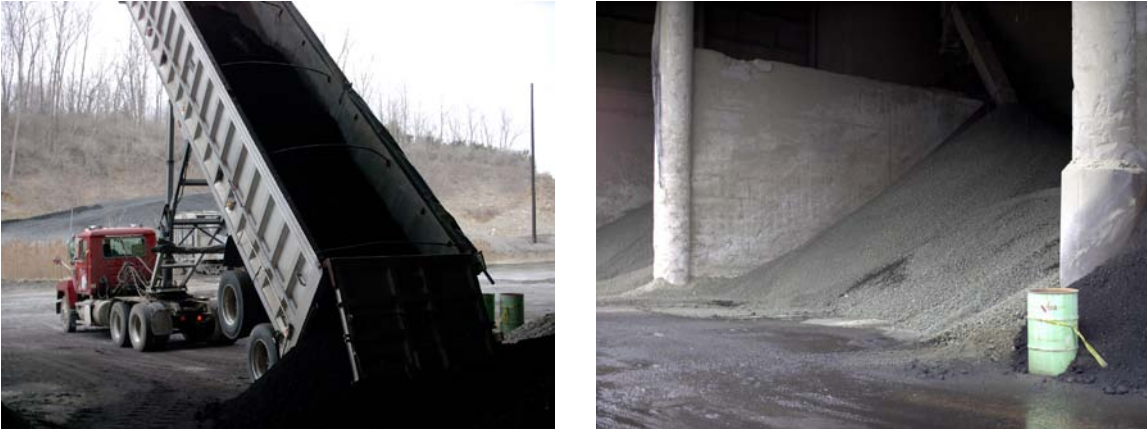
Figure 9. Prep-waste trucks being unloaded in covered storage at Greencastle plant
