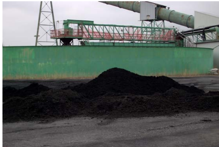
Figure 7. Coal prep-waste being spread out at drying site
