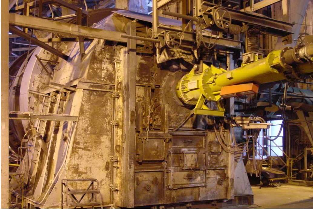
Figure 7. Prep-Waste/Regular Fuel Blend Introduced (yellow pipe) into Kiln
