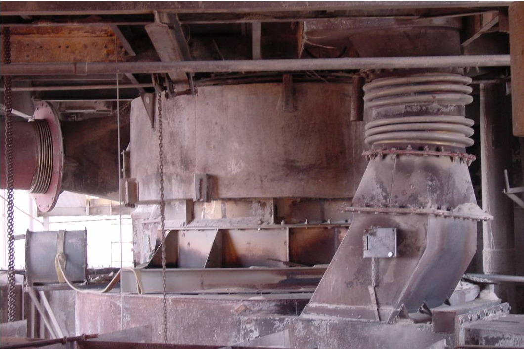
Figure 6. Prep-Waste and Regular Fuel Blend Introduced into Precalciner
