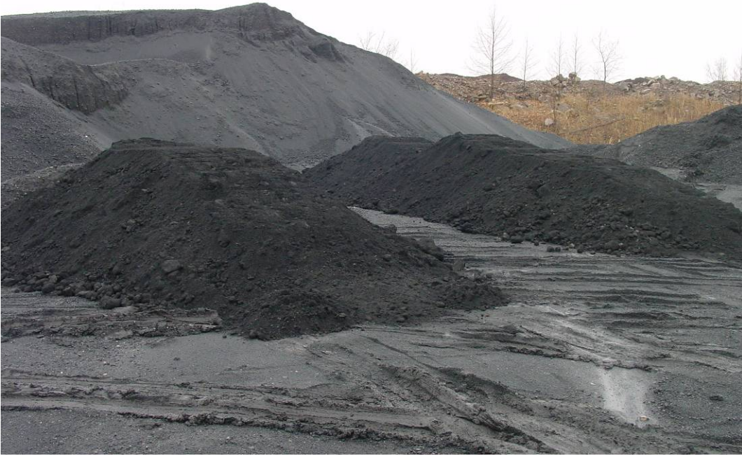
Figure 5. Prep-Waste (dark piles) Unloaded in Open at Cape Girardeau Plant for Air-Drying
