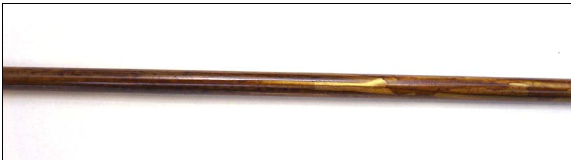
Figure 13: ABPBI-coating on Ceramic Porous Support.
