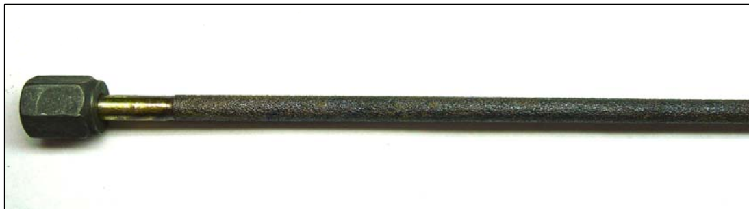
Figure 12: ABPBI-coating on Porous Stainless-steel Membrane.
