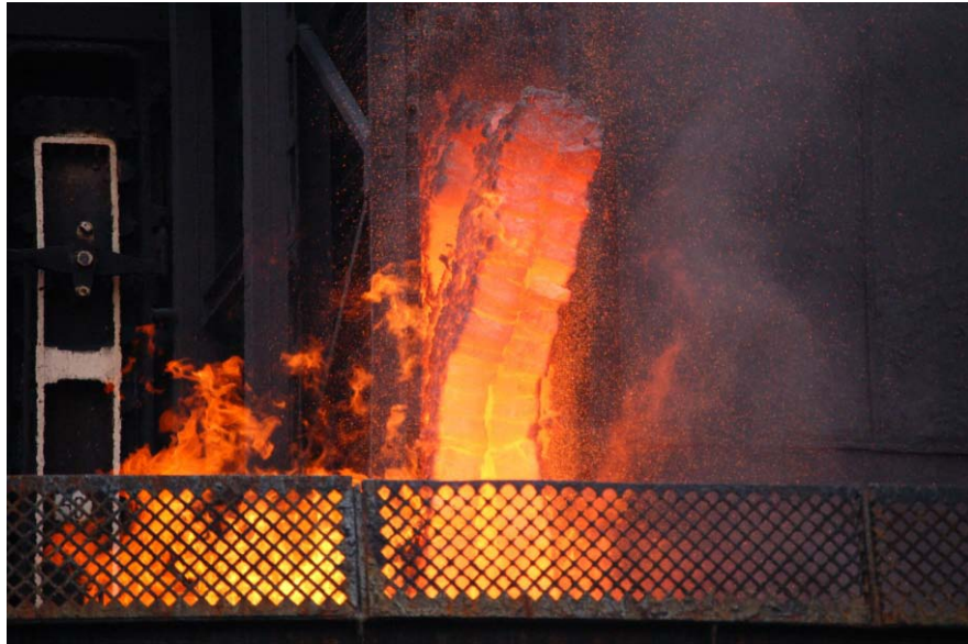
Figure 2: Coke in a Slot Coking Oven
